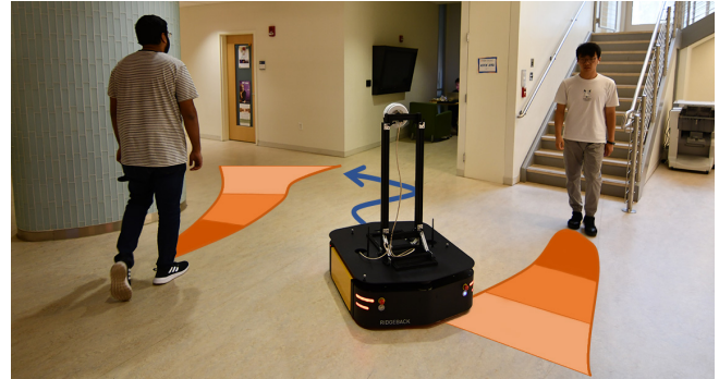
Fig. 1. Pictorial representation of the motivation behind this work. Our proposed approach computes temporal stochastic reachable sets and plans motion that proactively accommodates human intentions.
