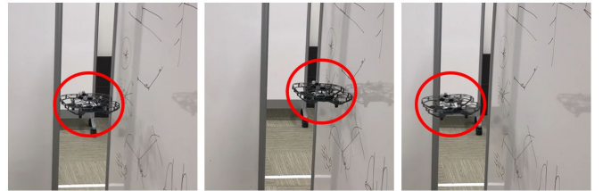
Fig. 8. A quadrotor detecting a collision and recovering from the crash site.
